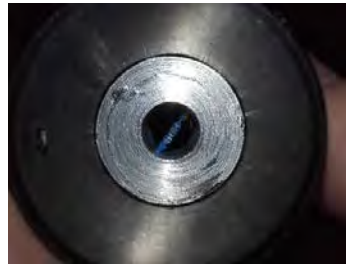
Figure 5 and 6. The detector, a 100 kOhm resistor is in the line of sight /in the focus, the other 3 resistors of the Wheatstone bridge are in the aluminum ring. The ring is placed in a 1.25 inch optical element replacing a Barlow lens
