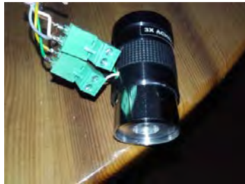
Figure 5 and 6. The detector, a 100 kOhm resistor is in the line of sight /in the focus, the other 3 resistors of the Wheatstone bridge are in the aluminum ring. The ring is placed in a 1.25 inch optical element replacing a Barlow lens
